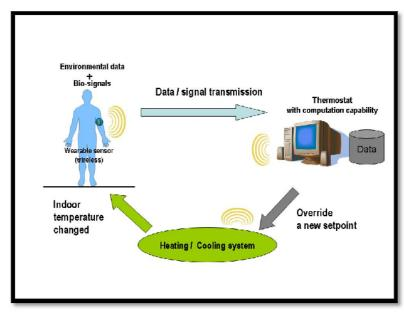
control of local heating and cooling units to meet user-preferred indoor temperatures instead of overheating or over cooling spaces, whether occupied or unoccupied.
